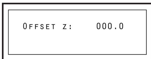
Use the supplied screwdriver to calibrate point 1. One rotation is 0.5 mm. For an offset of 0.7 mm rotate the screwdriver 1.5 turns.
