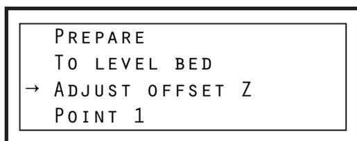
Place a piece of paper between the nozzle and heated bed and adjust the offset until the paper gets stuck between nozzle and heated bed
