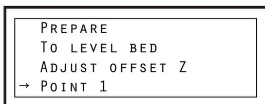
Adjust the height of the printhead with the option "Adjust offset Z"
