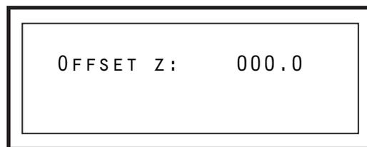
When the calibration of point 1 is complete put back the "offset Z" to 000.0 and move on to the next point.
